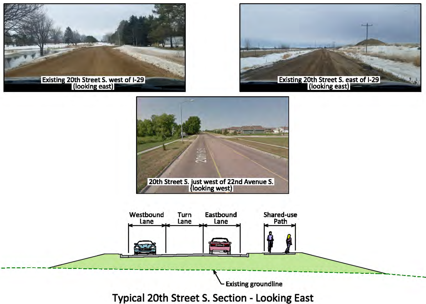
Figure 2-1. 20th Street South Typical Section
